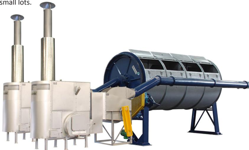
The new driers have two separate heat exchangers, one for each drying chamber of equal volume. This allows for the full flexibility of using the two half-drums in a completely independent manner, for different coffees at different drying stages and with different hot air and temperature requirements. Of course, the two half-drums can also be used with the same type of coffee if the need arises.
