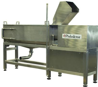
The latest addition to Pinhalense's cocoa line, the **mucilage remover**, was designed to shorten rather than to replace fermentation. Beans that go through this machine ferment for a shorter time – it saves one or two days – and dry faster without quality losses. It can be used in conjunction with the Pinhalense machines that transfer cocoa beans mechanically between fermentation boxes.
